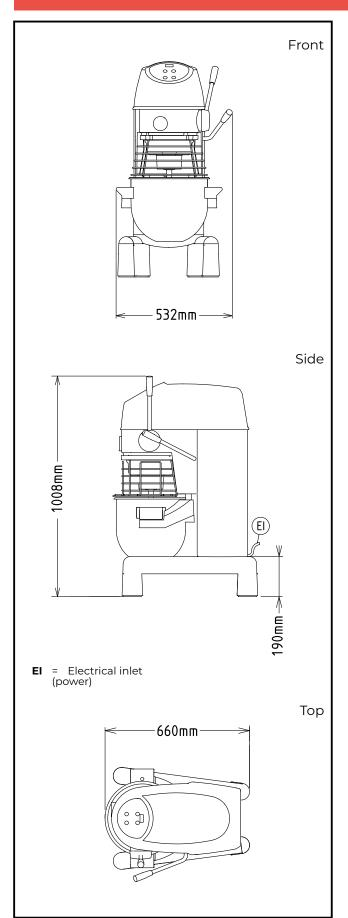
Electric 200-240/380-415 V/3 ph/50 Hz 9.75 kW 20.75 kW 20.75 kW
